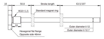
Option: Pressure-resistant outer pipe with flange, outer diameter 12mm/12.7mm
